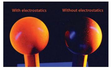
The black knob on the left was sprayed with fluorescent dye and with the electrostatic system turned *on*. However, the knob on the right was sprayed with the electrostatic system turned *off*. The spray coverage is so uneven that the back side of the knob remains untouched and is actually able to reflect the evenly-coated electrostatic knob.
